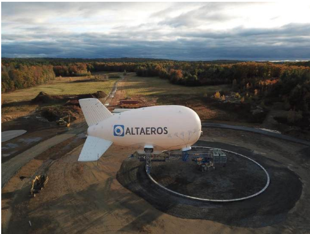
ST-200 aerostat docked at its fixed-base ground station. Source, both photos: Altaeros Energies (circa 2019)
