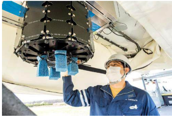
(L) The cylindrical phased-array antenna, and (R) antenna as installed in the payload bay in the Altaeros ST-Flex tethered aerostat. Source: SoftBank (2022)
