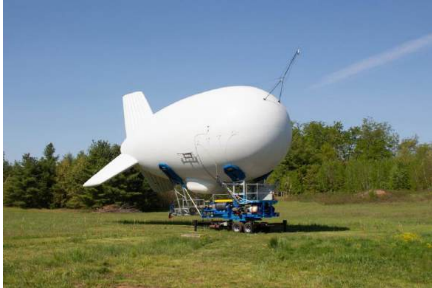
ST-Flex docked on its mobile ground station. Source: Altaeros
