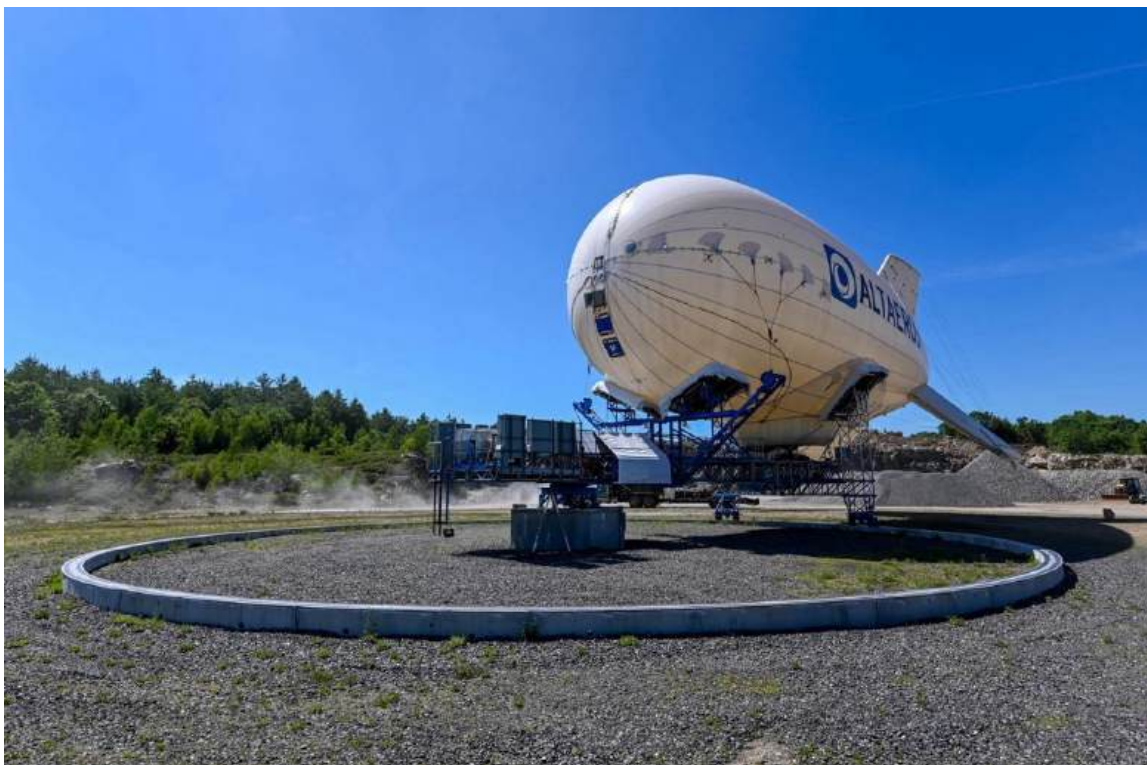
ST-300 aerostat docked at its fixed base. Source: Altaeros Energies
