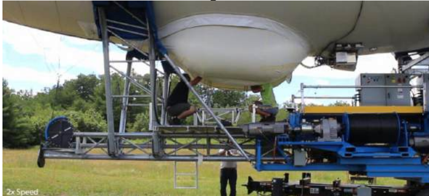
ST-Flex ground station includes a work platform that provides easy access to the payload pod attached under the gas envelope. Source: Screenshot from Altaeros video
