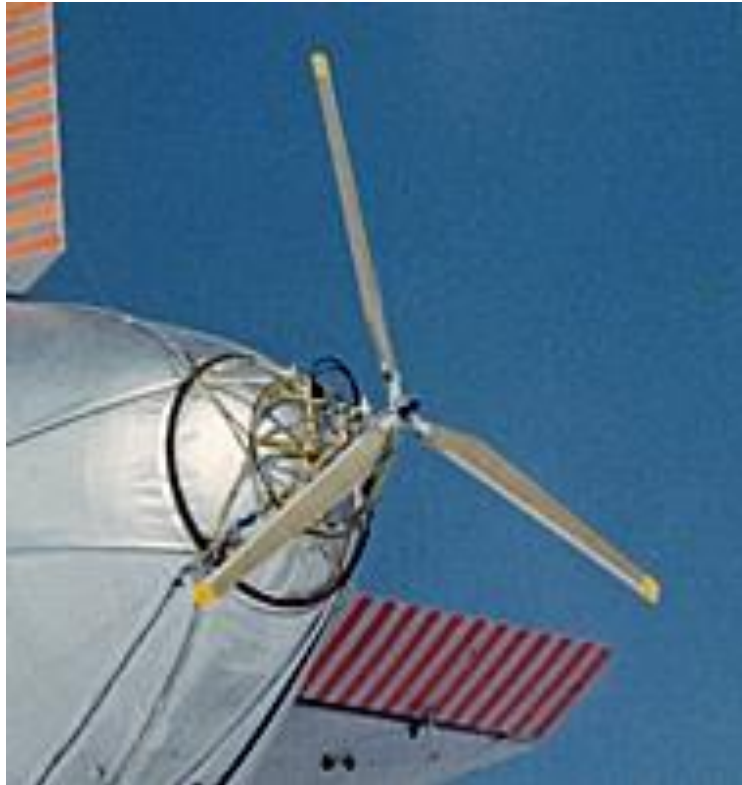
Closeup of the Silent Joe II stern propeller, the gimbal mount, the support rings and the Vee-battens. Source: Adapted from NAA Noon Balloon, #111 (2016)
