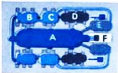
ATOMIC POWER PLANT A. SHIELDED PILE AND HEAT EXCHANGER B. HIGH PRESSURE TURBINE C. LOW PRESSURE TURBINE D. ELECTRIC GENERATOR E. STEAM CONDENSER F. CONTROL STATION
