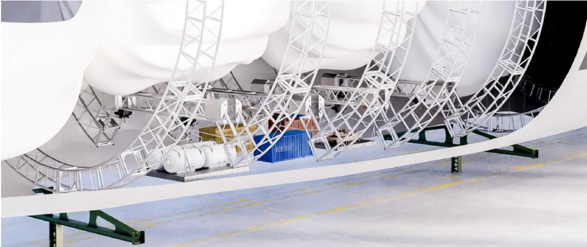
A closer look at the transverse rib structure of the hull reveals how the cargo bay is framed by trusses that bridge the bay and support the suspended cargo loads. Source: Airship Industries (circa Oct 2024)
