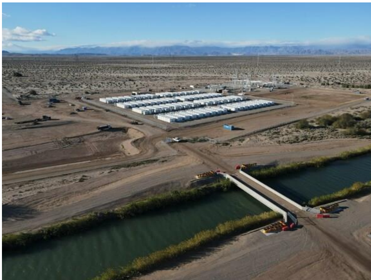
Aerial Photo of the Westside Canal Energy Storage Project, which is a Lithium-ion battery energy storage system situated in the desert adjacent to an irrigation canal. At full build-out, it is expected to have a capacity of about 2,000 MW. Source: SDG&E
